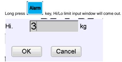
Press number keys to input high limit. Please take attention on the right unit show area. After input, press [OK], the Low limit window will pop-up. Use number keys to input low limit, then press [OK]. Note: The low limit value must lower than high limit value.
